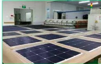
Solar panel lamination
