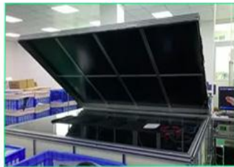
EL testing for foldable solar panel
