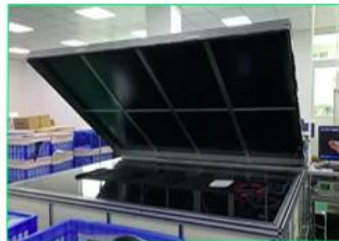
EL testing for foldable solar panel
