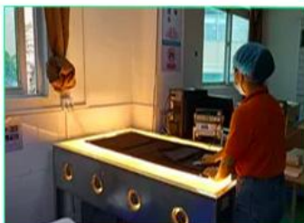
Power output testing for finished product
