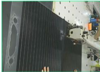
Sewing on the solar panels
