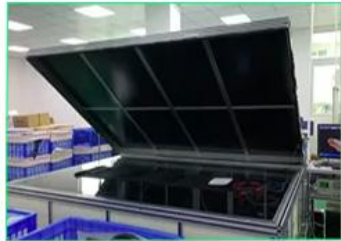
EL testing for foldable solar panel
