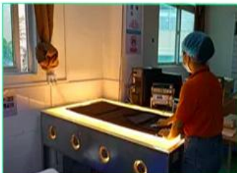
Power output testing for finished product
