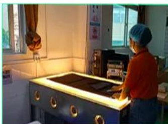
Power output testing for finished product
