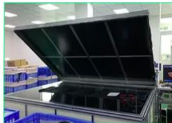
EL testing for foldable solar panel
