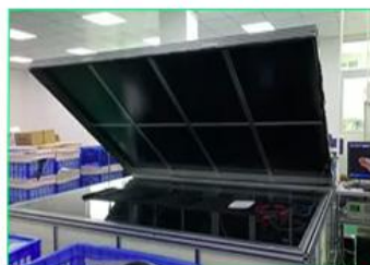
EL testing for foldable solar panel
