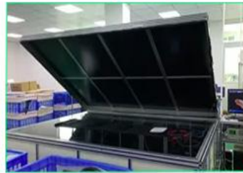
EL testing for foldable solar panel
